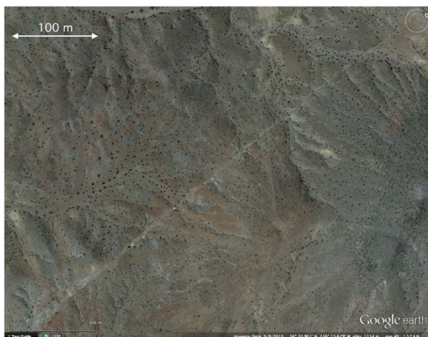
Fig. 2. Google Earth image of the Lavic Lake fault trace in the Mojave Desert in 2012, many years after the Hector Mine Earthquake (1999), which ruptured the surface. The fault trace is easily visible as a bright line through the landscape.
