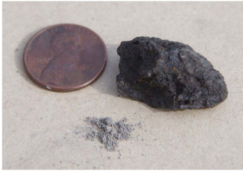
Fig. 4. Basalt pebble and a powdered fragment of it. The powder is brighter than the pebble itself.
